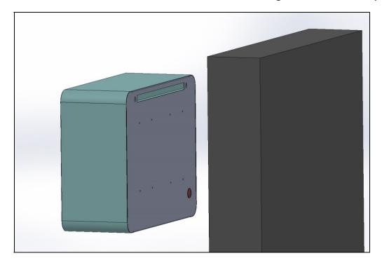
The slot in the back of the Onyx-W fits over the tab at the top of the mounting bracket. This will allow it to hang in place.
