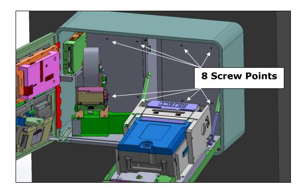
There are 8 screw points in the back of the chassis. It may be necessary to wiggle the machine to get some started. We recommend leaving the screws loose until they are all started and then tighten.
