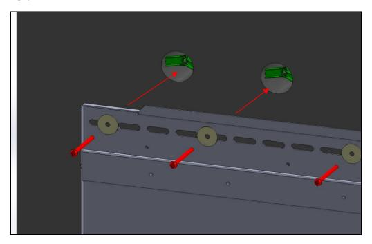
The elongated mounting holes provide flexibility to position the bracket. Make sure the bolts are flush when tightened.
