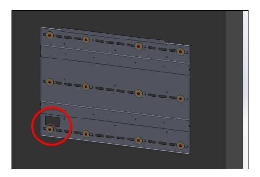
If you are going to route the cables internally through the wall, then you can cut out a section of the wall at this point in the mounting bracket. See red circle above.
