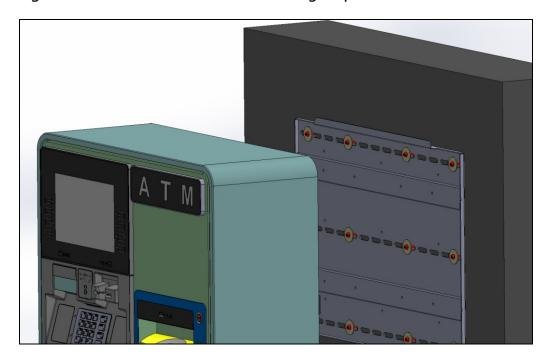
With the machine installed on the mounting bracket, you can now open the front of the machine to access the 8 screws that will be used to secure the machine to the bracket.
