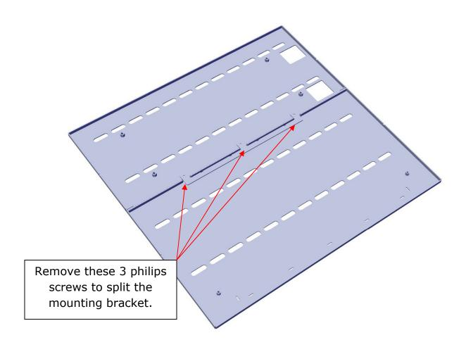
Below is the bracket used for mounting on countertops. There are several screw holes you can use to secure the machine to the top of the bracket. Then use the long slotted holes to mount the bracket to the counter.
