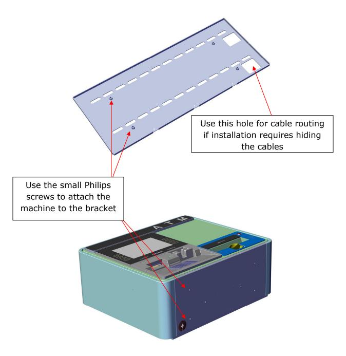
You will need to open the machine and swing out the printer to access 2 of these screws – the other 2 are inside the vault, behind the cash dispenser.
