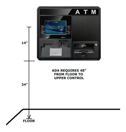
Note the photo above shows an Onyx-W 2K – the Onyx-W 1K has the same height from floor to function keys.
